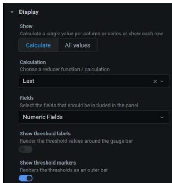
Figure 4.6 Additional gauge panel options for display
