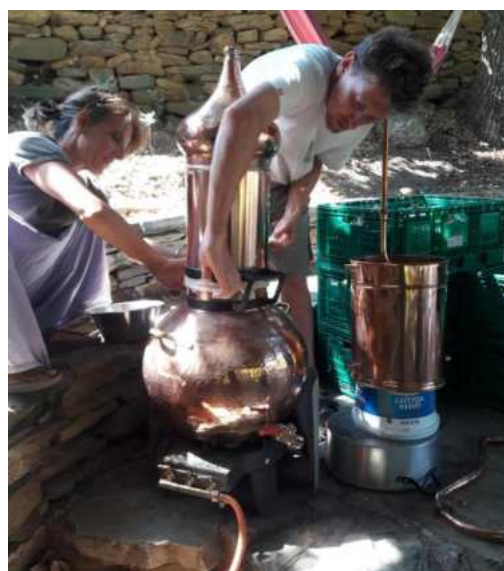
Figure 4.5. Assembling the distiller unit
