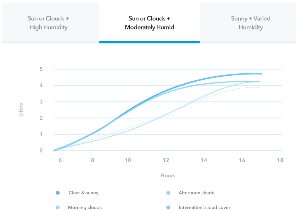
Figure 6.7 Water production capacity of one Hydropanel in optimal conditions
