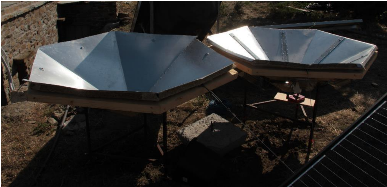
Figure 6.3 Setup of the 2 Water Flowers at HYDRO6, passive (left) and active (right)
