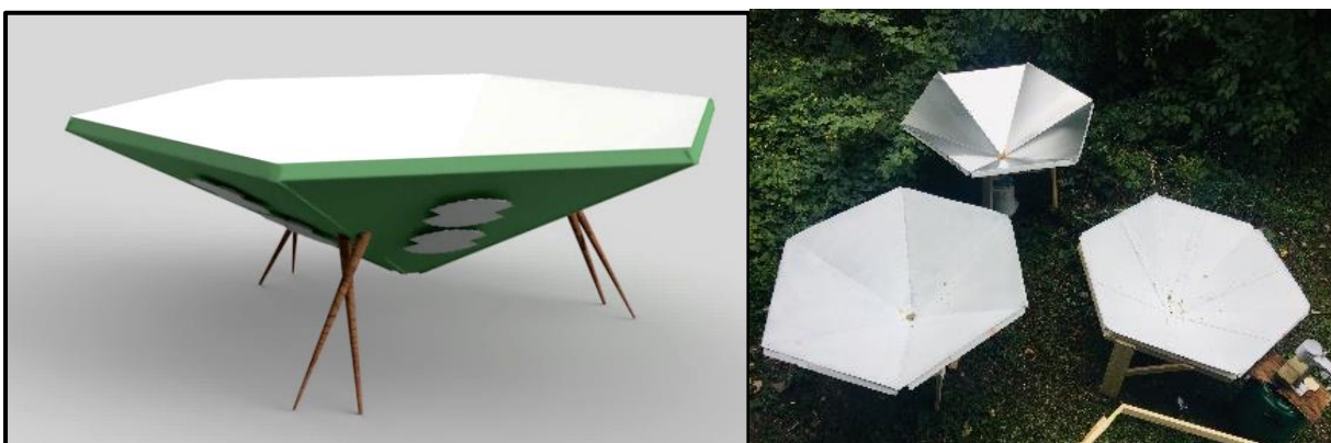
Figure 6.2 Sketch of cooled, coated Water Flower (left) and picture of the setup of all 3 prototypes
