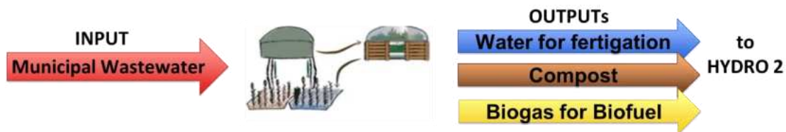
Figure 3.1 Simplified scheme of HYDRO 1 (derived from www.hydrousa.org/ )
