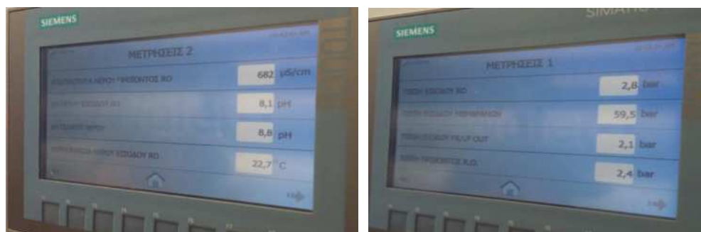
Figure 3.4: Measurements of the desalination system in Tinos (pH, temperature, pressure, conductivity)
