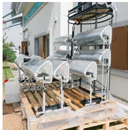
Figure 2.12: Mangrove Still desalination system on HYDRO 5
