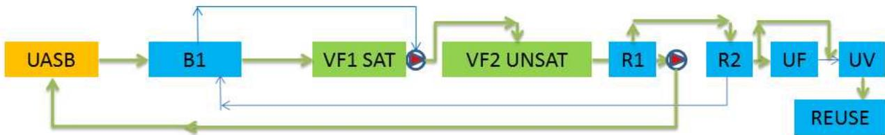
**Figure 2.10. Schematization of MODE 3 operation modes of full scale Lesvos system HYDRO1: green arrows represent the functioning treatment chain, while the blue arrows the turned off options within the operational mode.**
