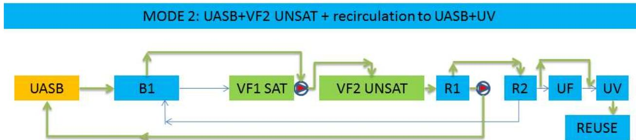
**Figure 2.9. Schematization of MODE 2 operation modes of full scale Lesvos system HYDRO1: green arrows represent the functioning treatment chain, while the blue arrows the turned off options within the operational mode.**
