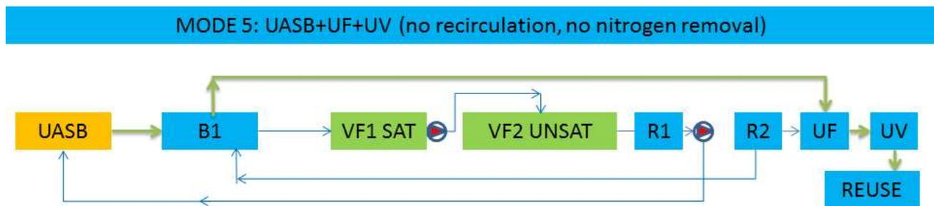
**Figure 2.12. Schematization of MODE 5 operation modes of full scale Lesvos system HYDRO1: green arrows represent the functioning treatment chain, while the blue arrows the turned off options within the operational mode.**
