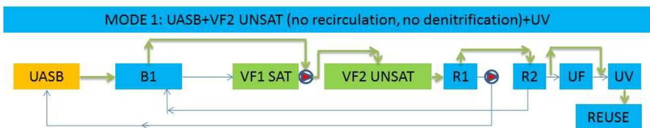
**Figure 2.8. Schematization of MODE 1 operation modes of full scale Lesvos system of HYDRO 1: green arrows represent the functioning treatment chain, while the blue arrows the turned off options within the operational mode.**
