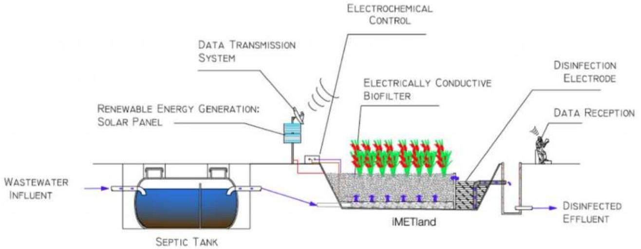
Figure 4.5. Schematization of IMET bio-electrified CW ([www.imetland.eu](http://www.imetland.eu))
