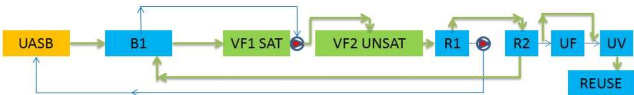
**Figure 2.11. Schematization of MODE 4 operation modes of full scale Lesvos system HYDRO1: green arrows represent the functioning treatment chain, while the blue arrows the turned off options within the operational mode.**
